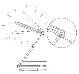
Loose lamp cap and the lever can be tightened with a screwdriver.
